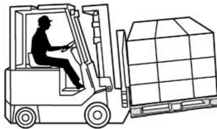
Dynamic load Max Uniformly distributed load that a pallet can carry when transported by forklift.
